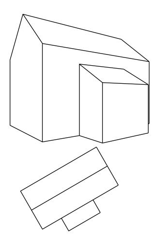
Either use a new height line to produce the windows or use the existing height line for the house gable and project round the walls of the house as shown below, care must be taken though.
