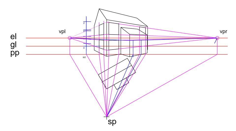
Note the top of the door and the top of the window are at the same height. Note where the blue perspective line for the top of the door passes through the intersection of the purple perspective line for the top of the window and the corner of the porch.
