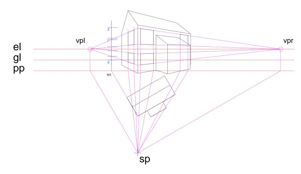
By continuing the technique of projecting in perspective round the walls, the position of the front door can be determined. See the projection lines in blue below. See next slide for clarification.
