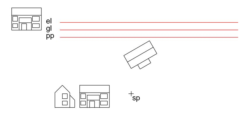
First project from the Spectator Point and determine the position of the LH and the RH vanishing points. Then decide which height lines should be produced.
