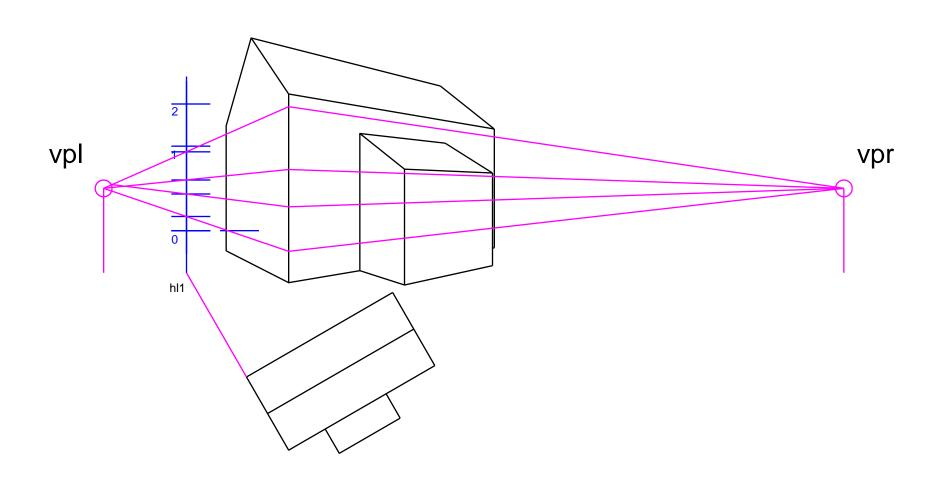
Having marked out the position of the windows on the plan, now view the windows from the spectator point and project these onto the perspective view.
