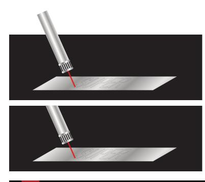
Apply a 24 degree rotation to the laser assembly. Move the laser assembly so that the laser beam touches the lower left part of the letter S.
